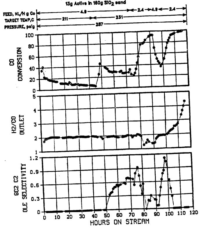
PLT 700A RUN 72 Co,Ru,Mn,Zr on MgO 6531-134 w/7.45% Co via eq. impreg 2:1 H<sub>2</sub>:00 in feed 13g Active in 160g SiO<sub>2</sub> sand
