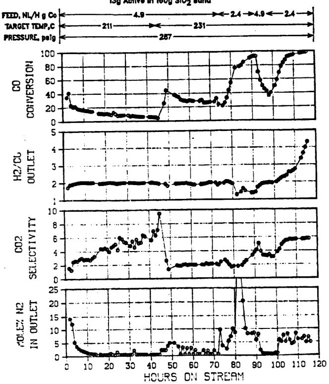
PLT 700A RUN 72 Co,Ru,Mn,Zr on MgO 6531-134 w/7.45% Co via eq. impreg 2:1 H2:CO in feed 13g Active in 160g SiO2 eand
