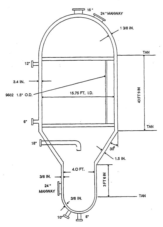
Design Conditions - Tube Side: 460 PSIG 550F; Shell Side: 580 PSIG 550F Metallurgy: Shell - SA516 GR70 with 1/8" C.A.; Tubes C.S. Chromized
