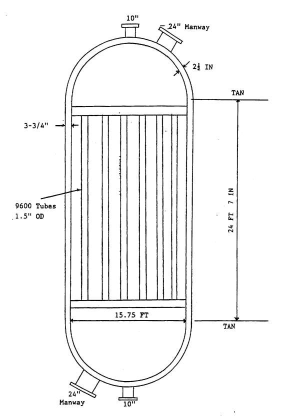
Design Conditions - Tube Side 875 PSIG 550F; Shell Side 650 PSIG 550F Metallurgy: Shell - SA516 GR70 with 1/8" C.A.; Tubes C.S. Chromized
