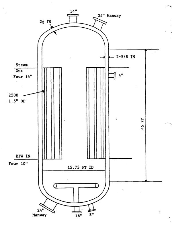
Design Conditions - Tube Side-580 PSIG 550F; Shell Side 460 PSIG 550F Metallurgy: Shell - SA516 GR70 with 1/8" C.A.; Tubes C.S. Chromized
