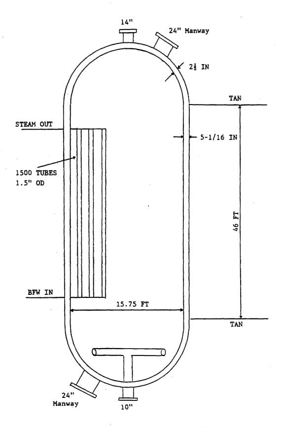
Design Conditions - Tube Side 580 PSIG 550F; Shell Side 875 PSIG 550F Metallurgy: Shell - SA516 GR70 with SS304 Cladding Tubes SS304
