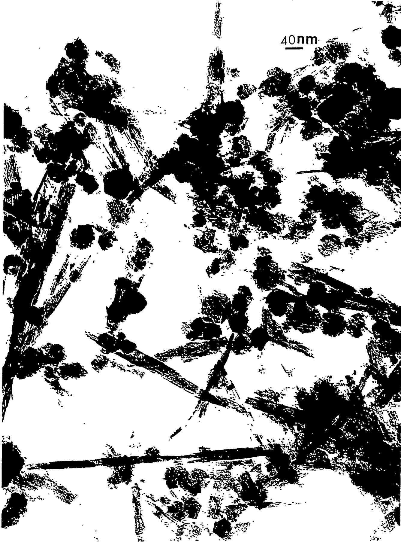
Figure IV.2.14. A typical electron micrograph from the L5 sample. Note the disappearance of large, thin hexagonal crystals with holes and the appearance of more number of dense spherical or hexagonal particles as well as the fiber-like \gamma -FeOOH particles.
