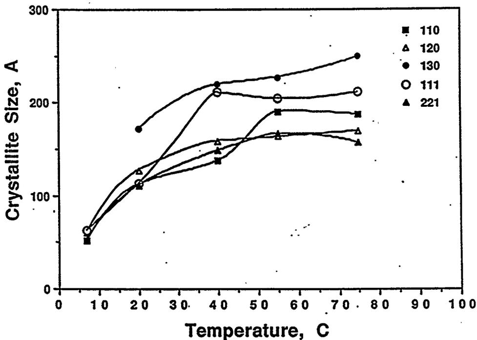
Figure IV.4.8. Crystallite size vs oxidation temperature at different crystalline planes. -■- 110 plane, -△- 120 plane, -●- 130 Plane, -○- 111 Plane, -▲- 221 plane.
