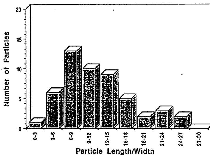
Figure IV.4.21. Length/width ratio distribution for  $\alpha$ -FeOOH particles prepared at 55°C.
