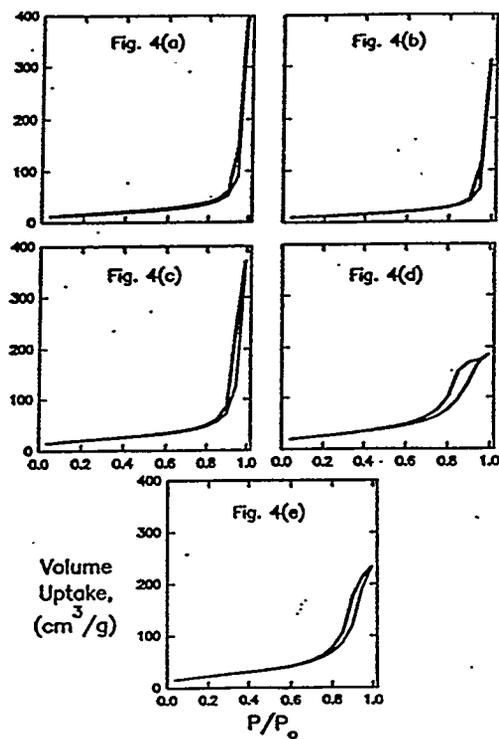
Figure IV.4.4. Nitrogen adsorption and desorption isotherms for the  $\alpha$ -FeOOH samples prepared at different oxidation temperatures. (a) 7°C, (b) 20°C, (c) 40°C, (d) 55°C, and (e) 75°C. - + - Adsorption and -●- Desorption.
