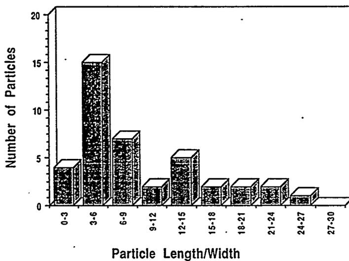
Figure IV.4.22. Length/width ratio distribution for  $\alpha$ -FeOOH particles prepared at 75°C.
