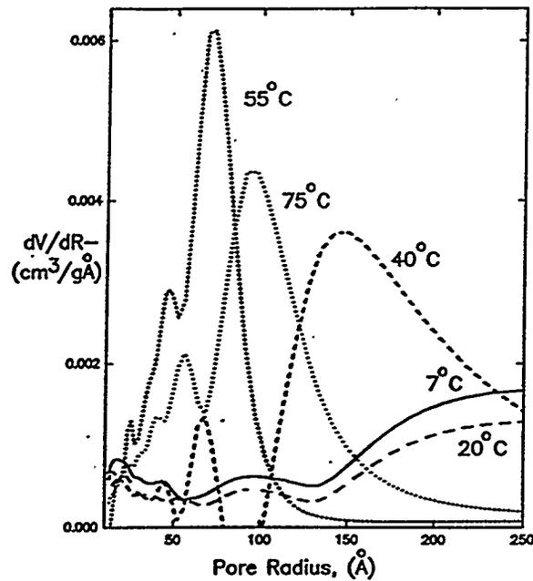
Figure IV.4.5. Effect of oxidation temperature on the pore size distributions for  $\alpha$ -FeOOH samples prepared at different temperatures. (a) 7°C, (b) 20°C, (c) 40°C, (d) 55°C, and (e) 75°C.
