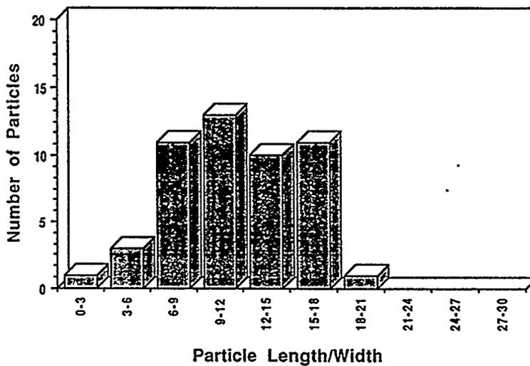
Figure IV.4.20. Length/width ratio distribution for  $\alpha$ -FeOOH particles prepared at 40°C.
