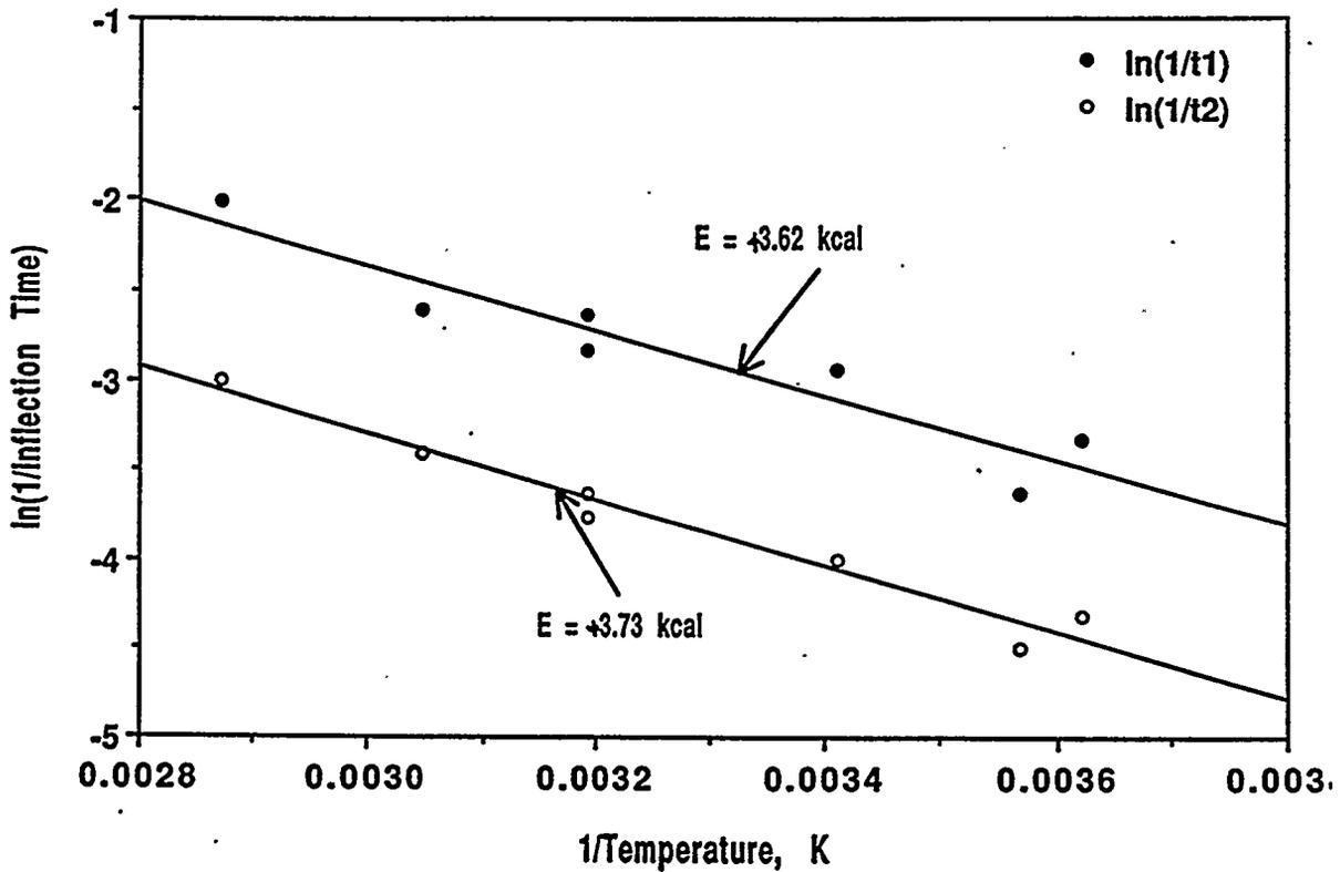
Figure IV.4.2. ln (inflection) times vs 1/T. (a)  $\bullet$  - t<sub>1</sub> and (b)  $\circ$  - t<sub>2</sub>.
