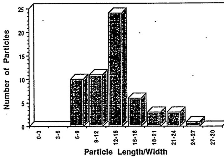
Figure IV.4.19. Length/width ratio distribution for  $\alpha$ -FeOOH particles prepared at 20°C.
