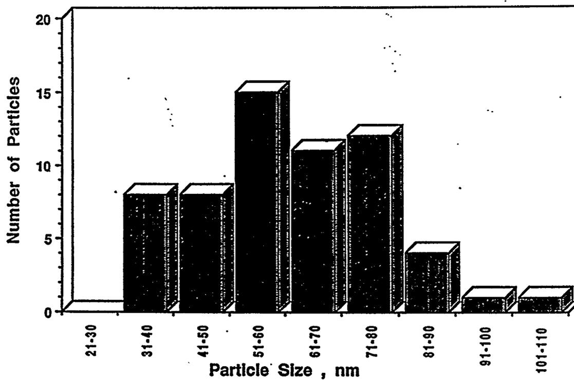
Figure IV.4.12. Particle size distribution for the the Fe<sub>3</sub>O<sub>4</sub> sample.
