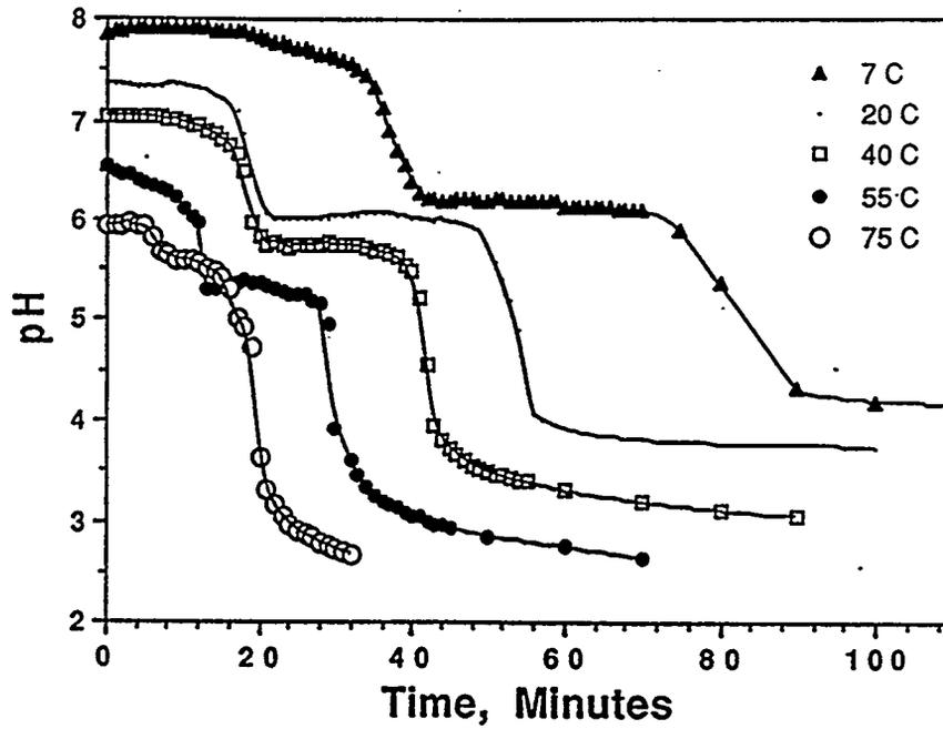
Figure IV.4.1. pH vs oxidation time during the oxidation of Fe(II) in aqueous solution with molecular oxygen. (a)  $\blacktriangle$  = 7°C, (b)  $\cdot\cdot$  = 20°C, (c)  $\square$  = 40°C, (d)  $\bullet$  = 55°C and (e)  $\circ$  = 75°C.
