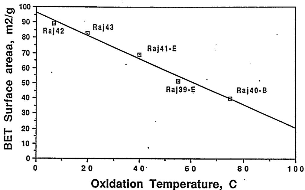
Figure IV.4.3. Effect of oxidation temperature on the BET surface area of  $\alpha$ -FeOOH samples.
