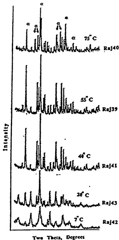
Figure IV.4.7. Oxidation of ferrous hydroxide aqueous suspension with molecular oxygen at different temperatures. (a) 7°C, (b) 20°C, (c) 40°C, (d) 55°C, and (e) 75°C.
