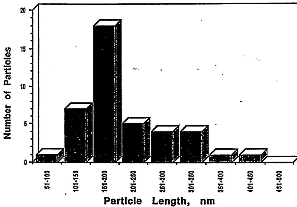
Figure IV.4.10. Particle size (length) distribution for  $\alpha$ -FeOOH sample prepared at 55°C.
