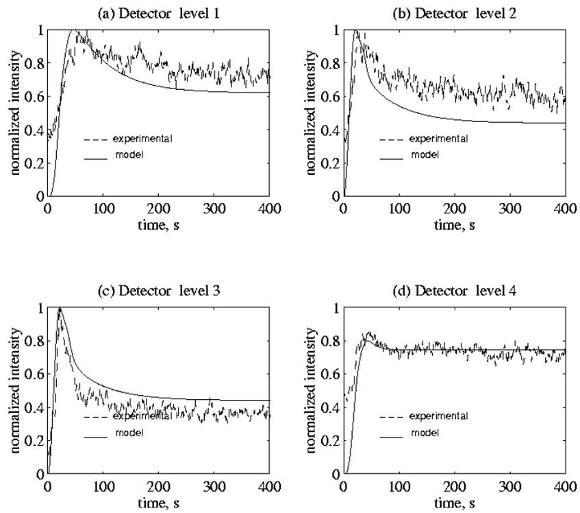
**Figure 2.18 Comparison of Model Prediction with Experimental Detector Responses for Center Injection at Level N2, Run 14.6**
