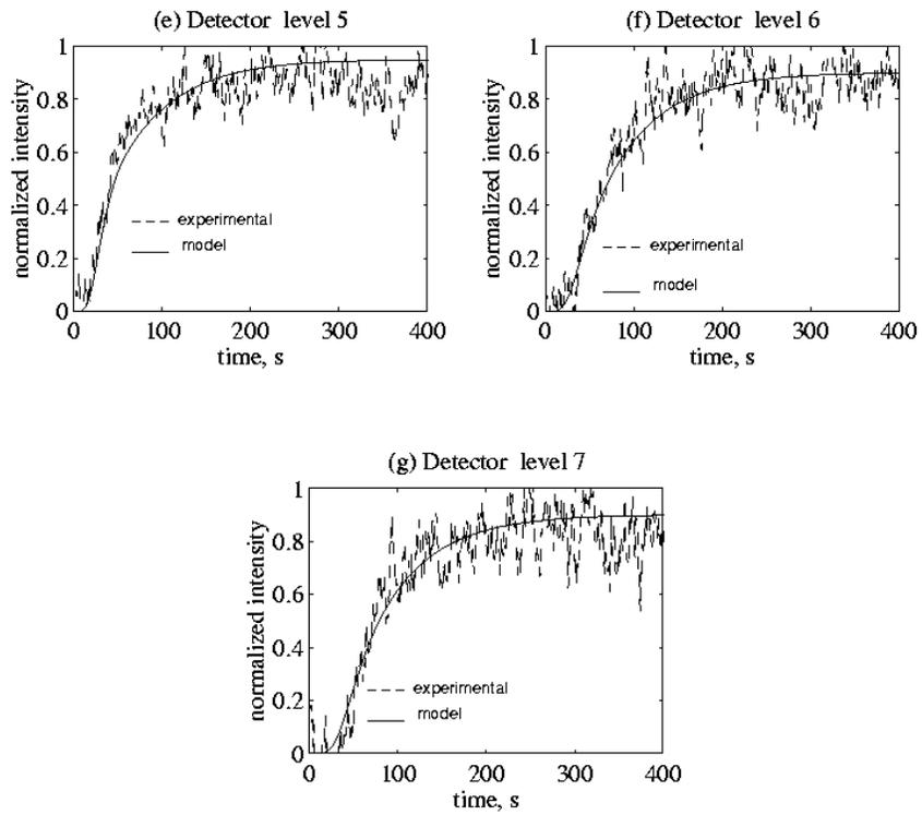
**Figure 2.19 Comparison of Model Prediction with Experimental Detector Responses for Center Injection at Level N2, Run 14.6**
