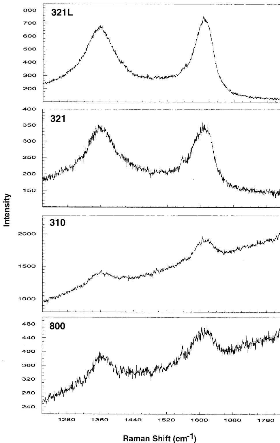
Fig. 47. Raman spectra (frequency range 1200-1800  $\text{cm}^{-1}$ ) for surfaces of 300-series stainless steel alloys and Alloy 800 after 1000-h exposure in a metal dusting environment at 593°C (1100°F).
