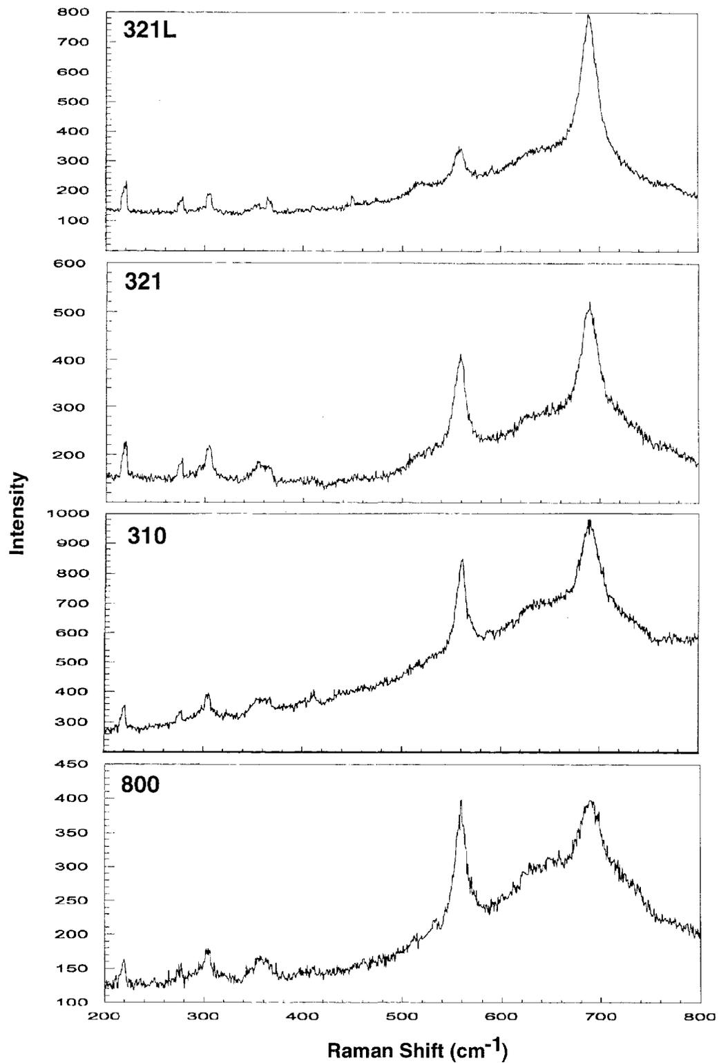
Fig. 46. Raman spectra (frequency range 200-800 cm<sup>-1</sup>) for surfaces of 300-series stainless steel alloys and Alloy 800 after 1000-h exposure in a metal dusting environment at 593°C (1100°F).
