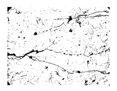
condensation. The second stress-chloride cracking failure was in the char-sampling line in a weld area between a 316 SS male connector and a 316 SS half coupling. This line had been fully wrapped with tape heaters and insulation and held at 600-650°F. Steam evidently condensed at some time, however, probably during a shutdown as a result of inadequate purging.
