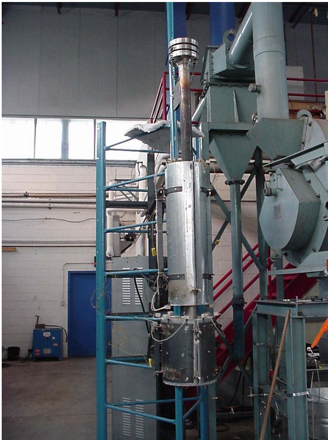
Figure 7: Assembled and Mounted Fluidized Bed Reactor, Furnace and Preheater
