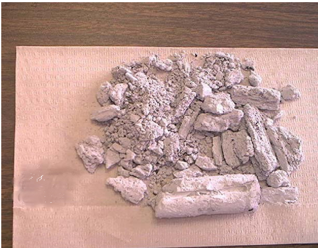
Figure 33: Solids of 1:7 \text{Fe}_2\text{O}_3 :CaO Mixture After One Hydrogen Generation Cycle
