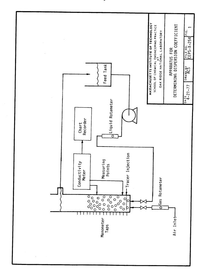
maintains a constant liquid level in the column. Sixteen water manometers are connected to ports at 8-cm intervals up the column beginning one centimeter above the distributor plate. A mercury manometer is connected to the air feed line to monitor the pressure drop through the column.
