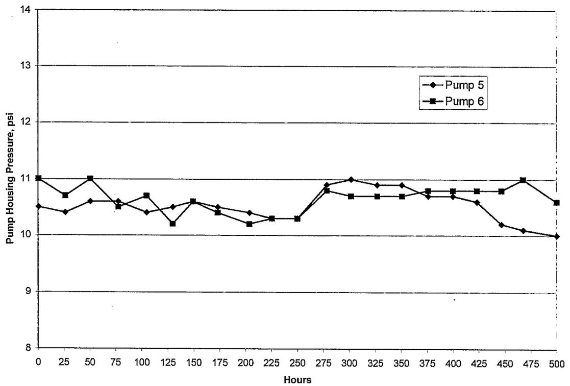
Figure A-12. Pump Test 3 - Pump Housing Pressures
