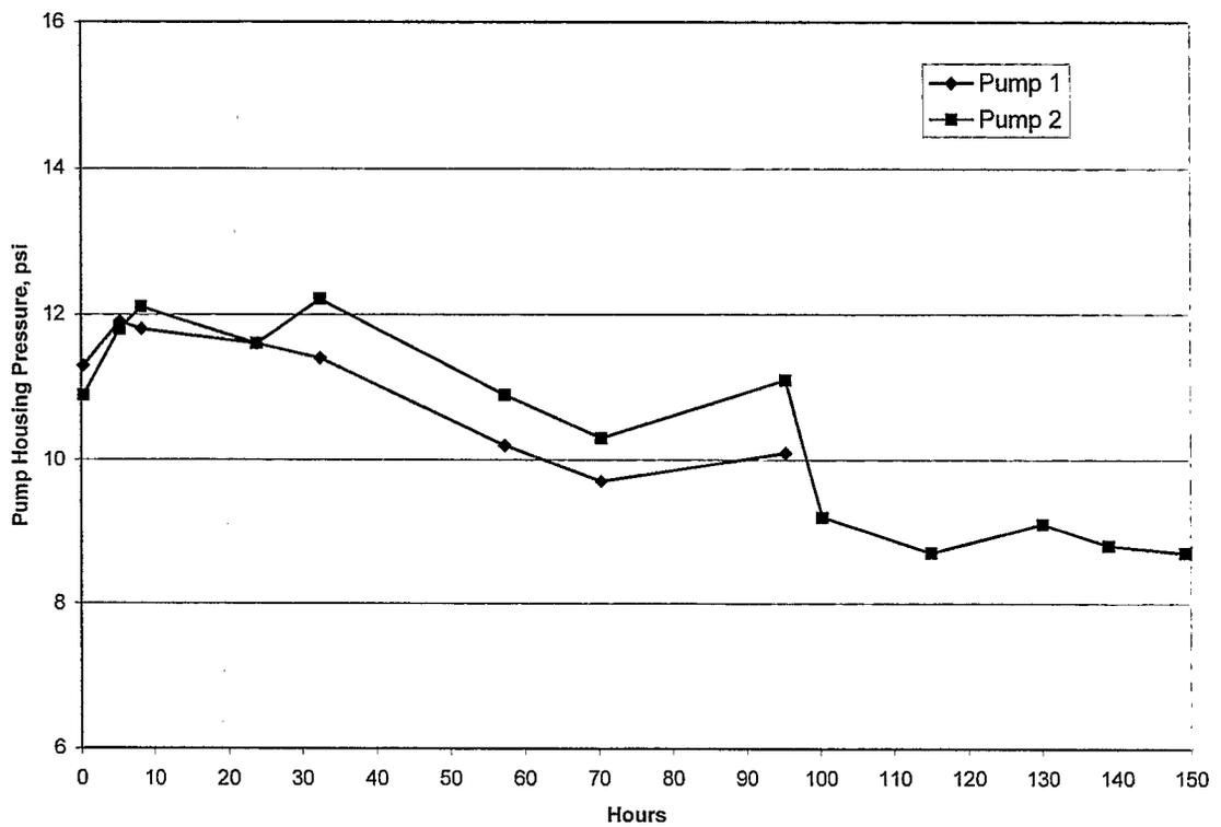
Figure A-4. Test 1 - Pump Housing Pressures
