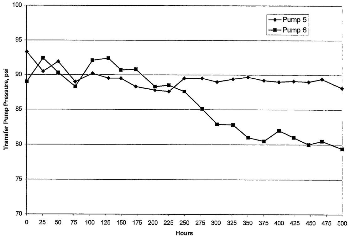
Figure A-11. Test 3 - Transfer Pump Pressures
