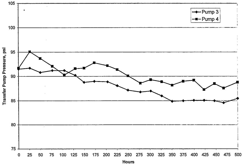
**Figure A-7. Test 2 - Transfer Pump Pressures**
