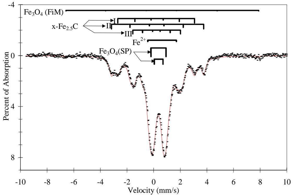
Fig 15. Mossbauer Spectrum of Fe-S-201 (10.7 % Fe/SiO<sub>2</sub>) after statistically designed experiments run #03
