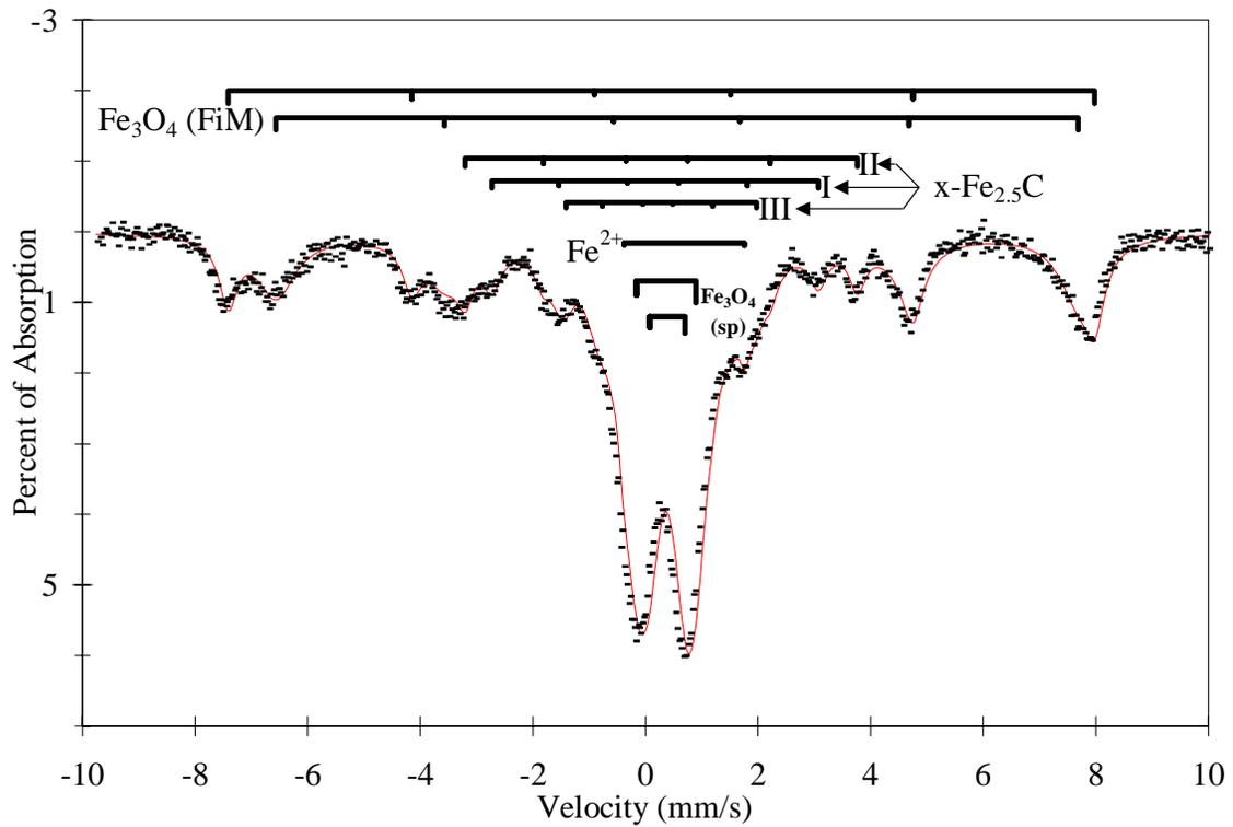
Fig 13. Mossbauer Spectrum of Fe-S-201 (10.7 % Fe/SiO<sub>2</sub>) after statistically designed experiments run #01
