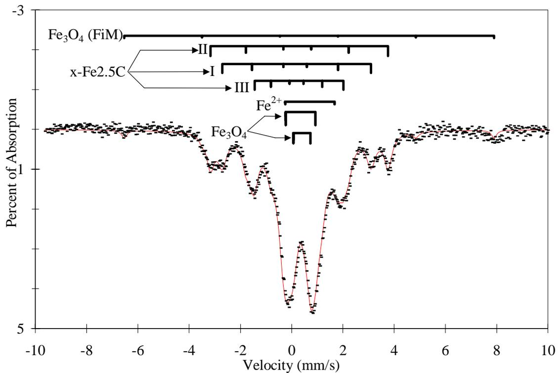
Fig 14. Mossbauer Spectrum of Fe-S-201 (10.7 % Fe/SiO<sub>2</sub>) after statistically designed experiments run #02
