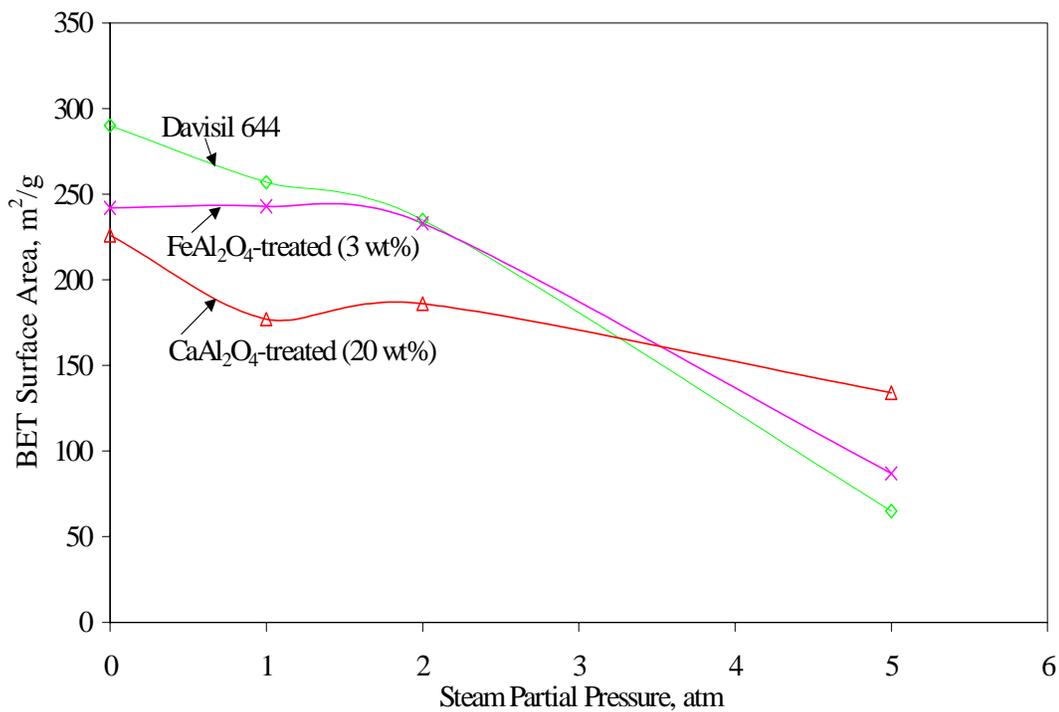
Fig 3. Hydrothermal Stability of Davisil 644 Silica support and FeAl<sub>2</sub>O<sub>4</sub> Modified Davisil 644 Support (72 h steam treatment at P<sub>total</sub>=10 atm, T=265°C, repeat every run) BET Surface Area Thermal Stability of Davisil 644
