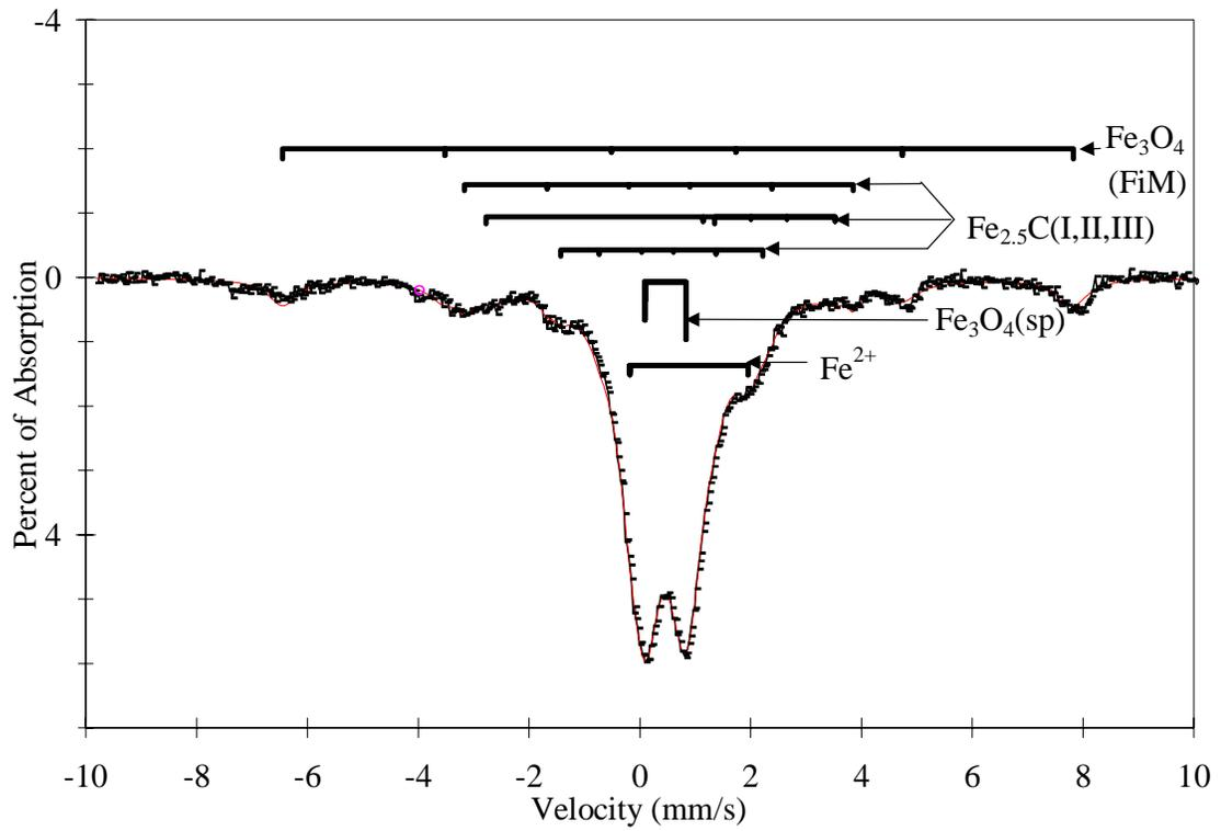
Fig 12. In-situ Mössbauer spectrum of Fe-S-207 after pretreated at 280°C, 1atm and H<sub>2</sub>/CO=1.
