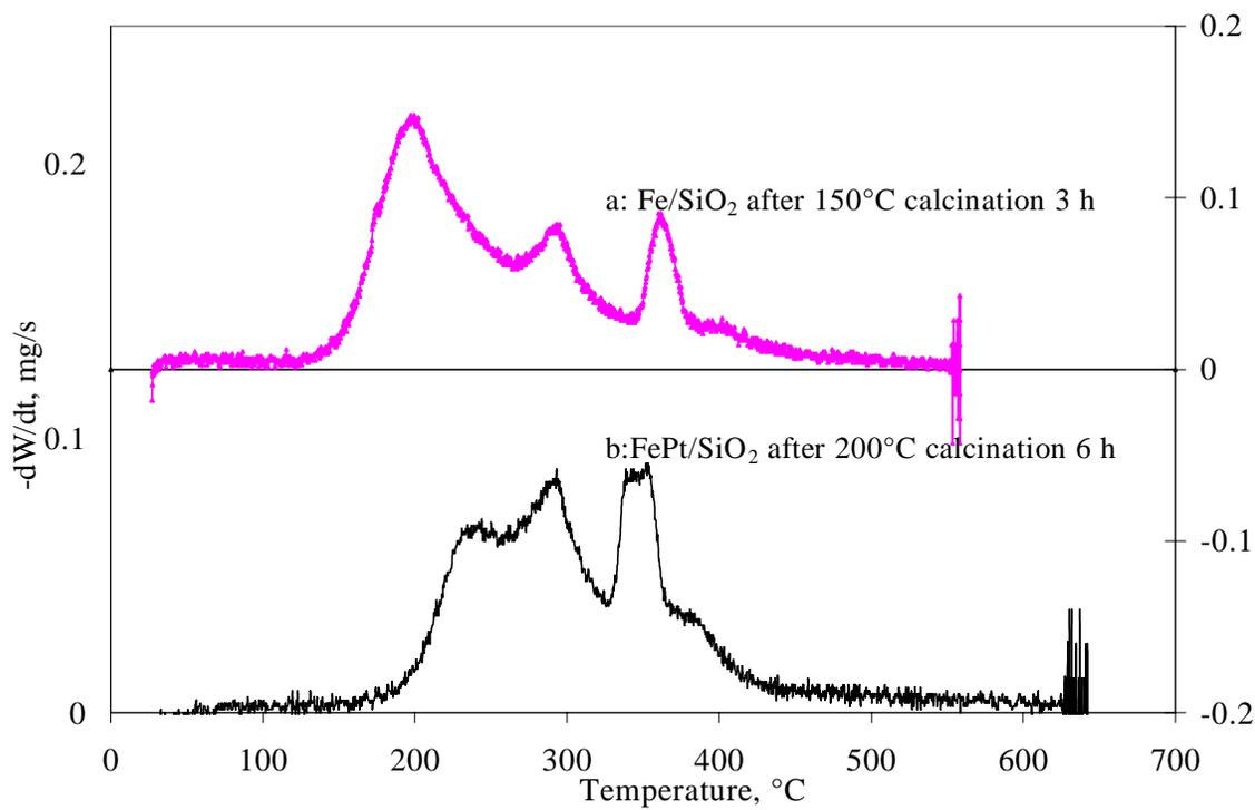
Fig 7. TPR of calcined Fe-S-207 and FePt-S-207
