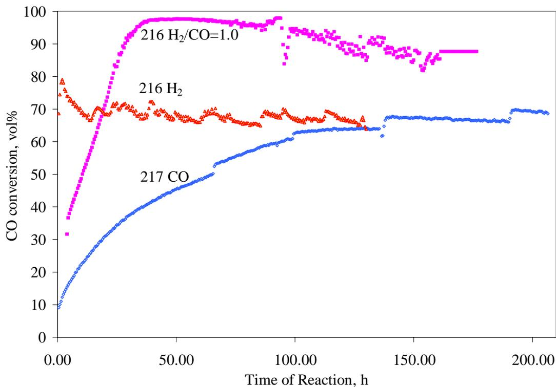
Fig 25. Pretreatment effects on FePtK-S-216 and FePtK-S-217
