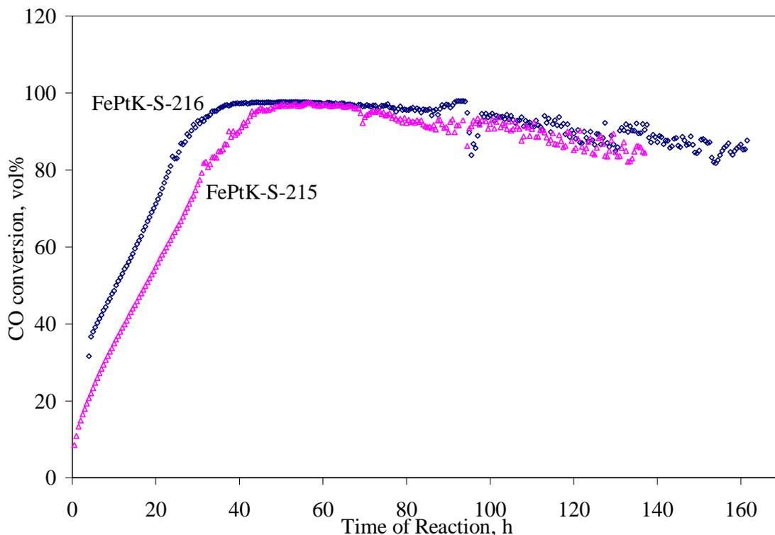
Fig 24. Repeatability of FePtK-S-215 and FePtK-S-216 fixed bed runs T=265°C, P=10 atm, Total Flow=64 sccm, H<sub>2</sub>/CO=1
