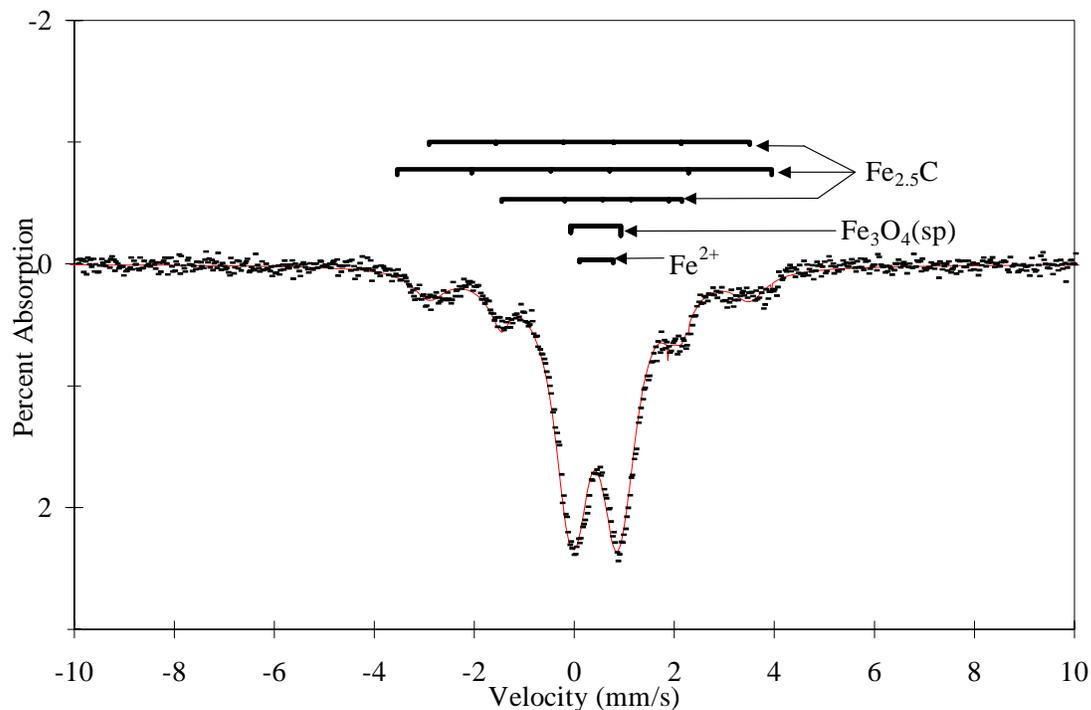
Fig 9. Fe-S-206 After 55hrs fixed bed test run
