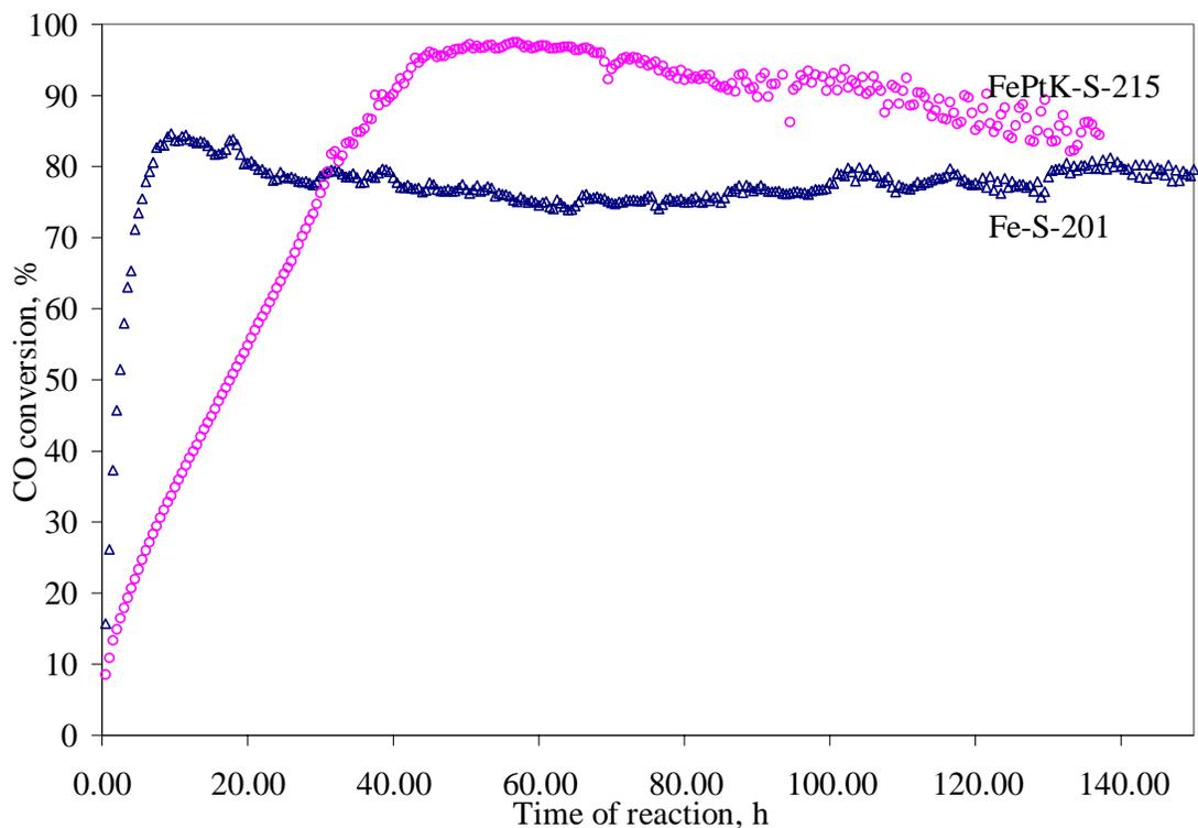
Fig 23. CO conversion of FePtK-S-215 compared with Fe-S-201 at 265°C, 10 atm, H<sub>2</sub>/CO=1
