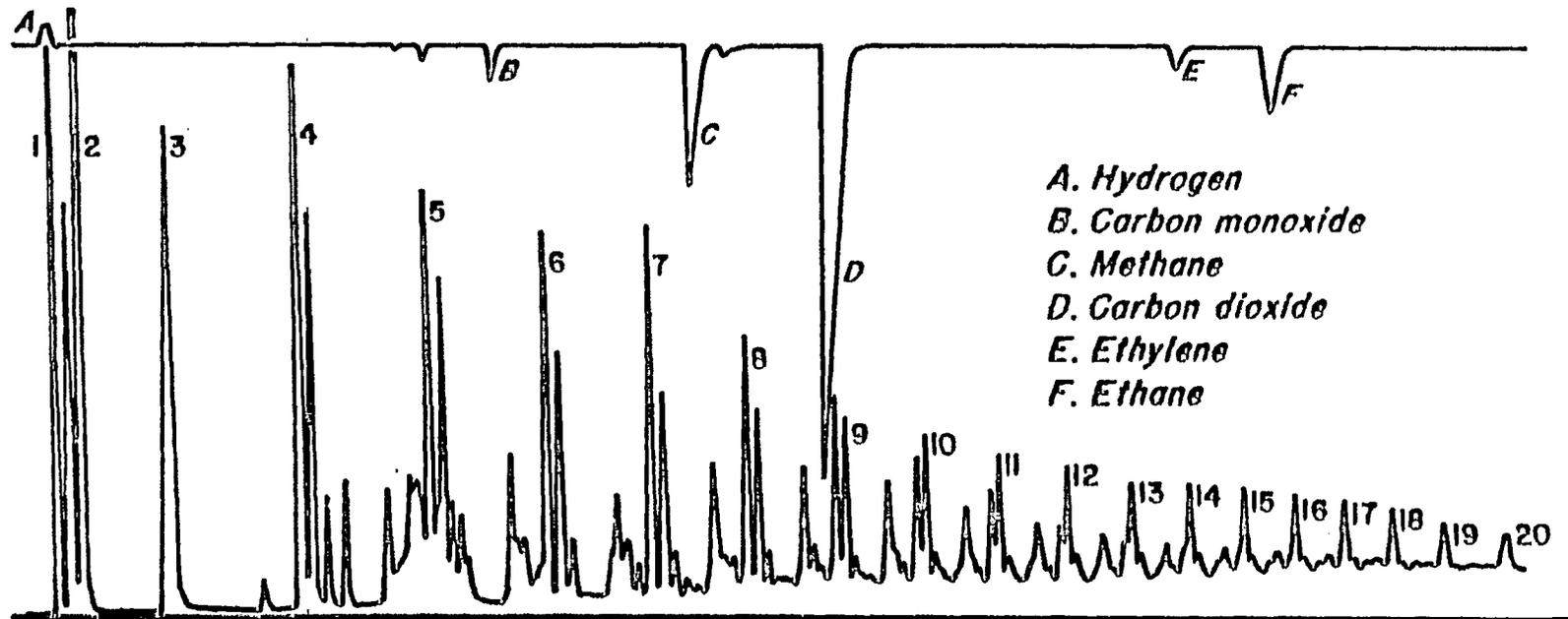
Figure 10- Gas chromatogram of Fischer - Tropsch Product . Peaks numbered 1-20 represent  $C_1$ - $C_{20}$  hydrocarbons as detected by FID. Peaks labeled A-F were detected on the TCD.
