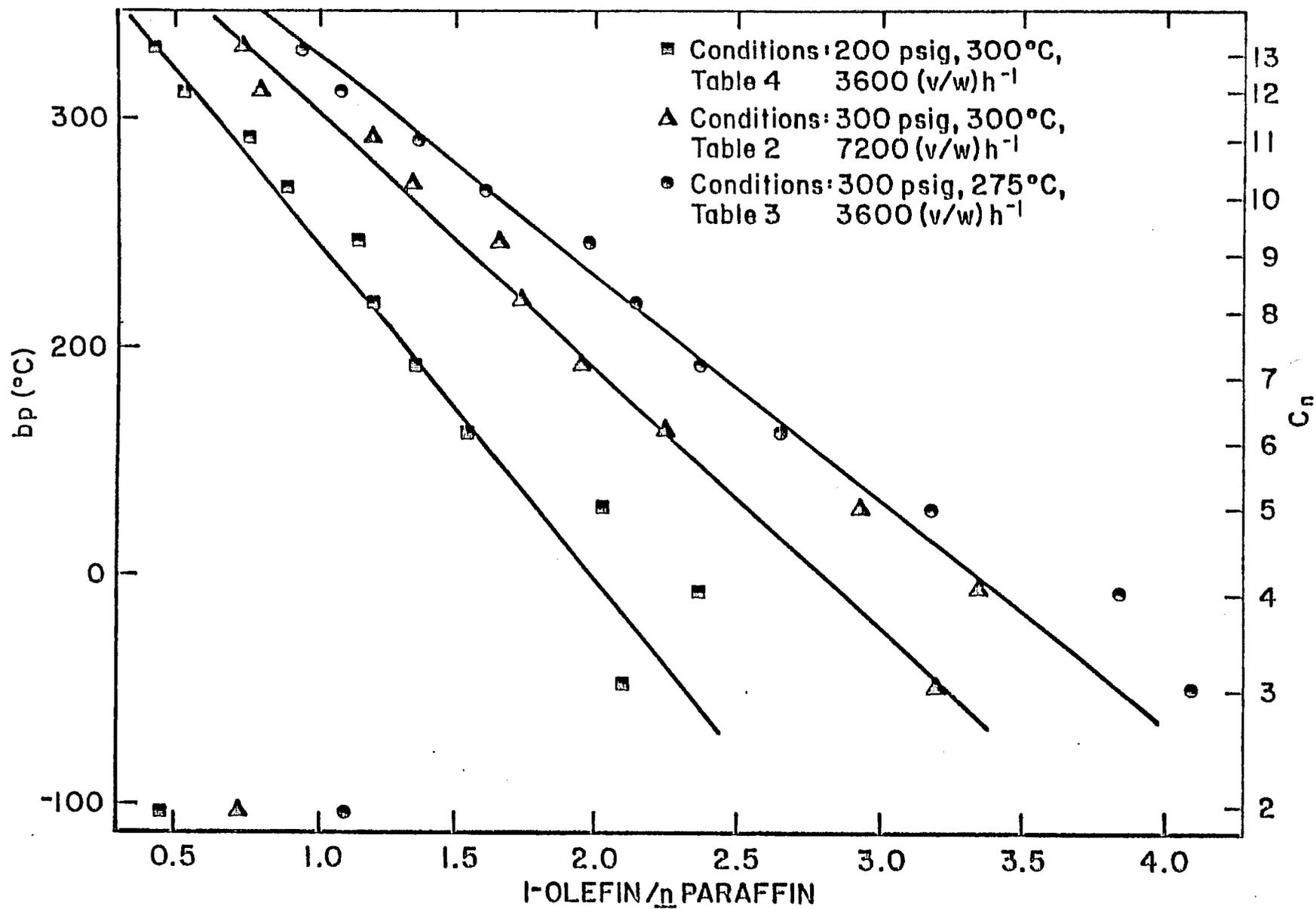
Figure 7-Comparison of I-Olefin/n-paraffin ratios to boiling points of olefins under different reaction conditions.
