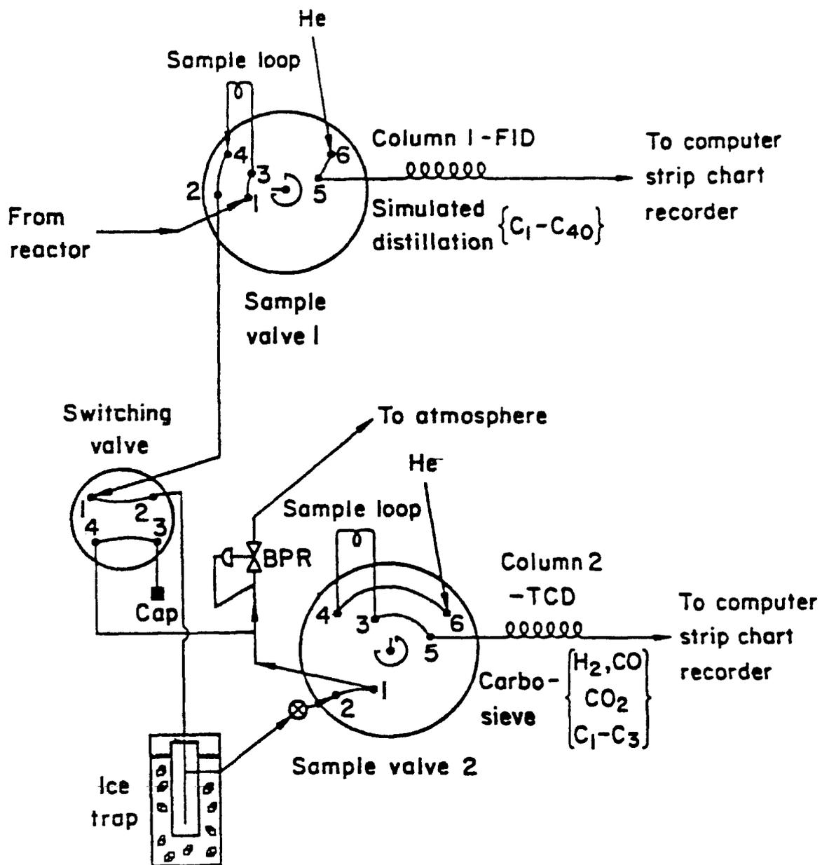
Figure 9 - Sample valve compartment.
