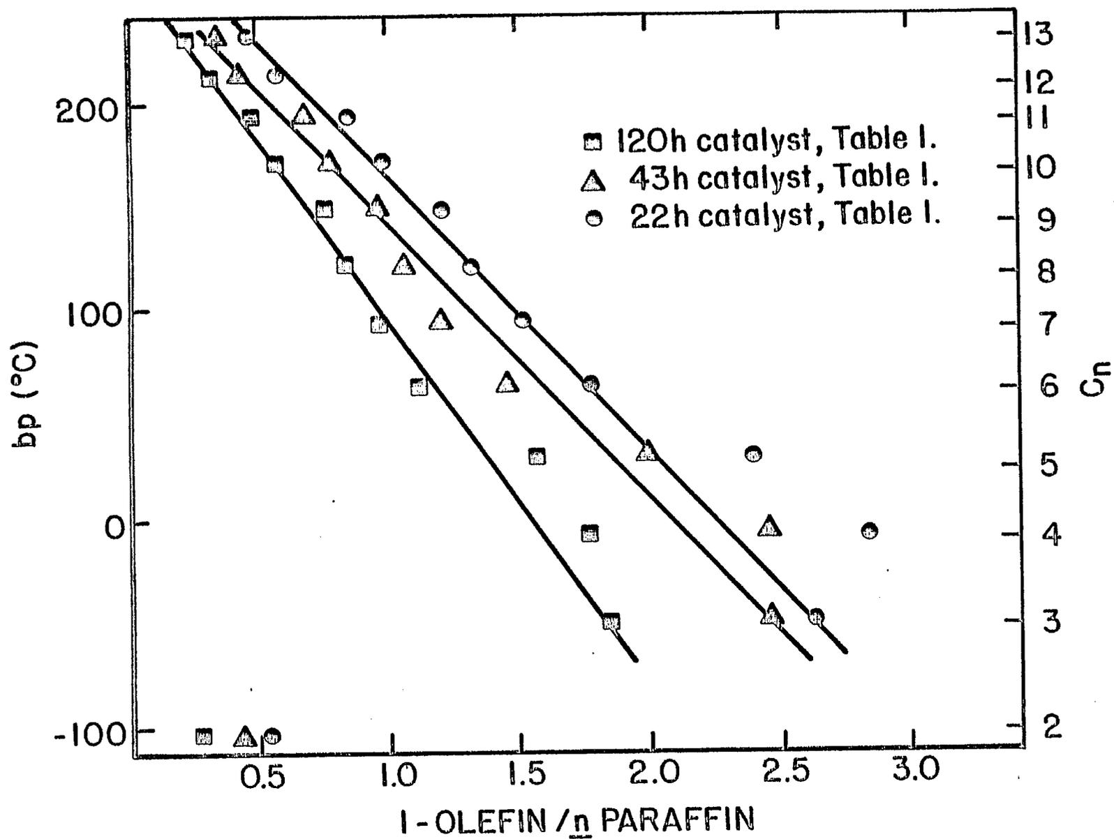
Figure 6 - Comparison of I-Olefin/ $n$ -Paraffin ratios to boiling points of olefins at different catalyst reaction times.
