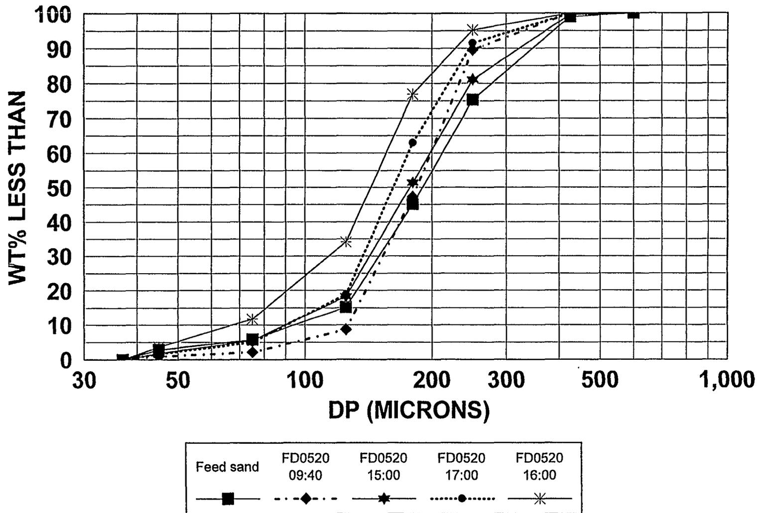
Figure 5.1.9-22 Feed Sand and PCD Solids Particle Size Distribution on November 4, 1996
