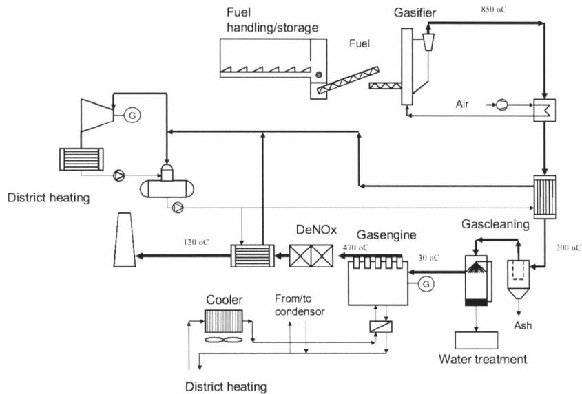
**Figure 4. Flow sheet of the 14.7 MW<sub>th</sub> BIVKIN-based power plant**
