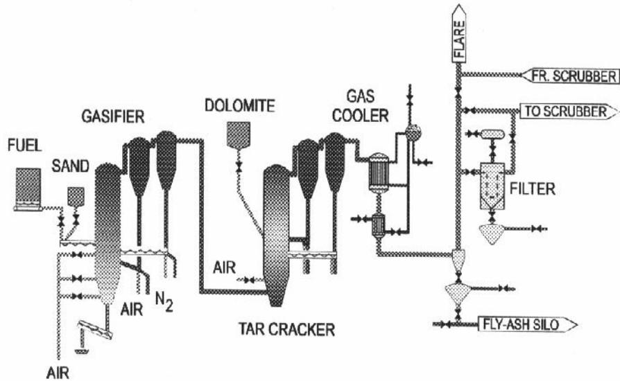
**Figure 13. TPS Pilot Plant with Tar Cracker**
