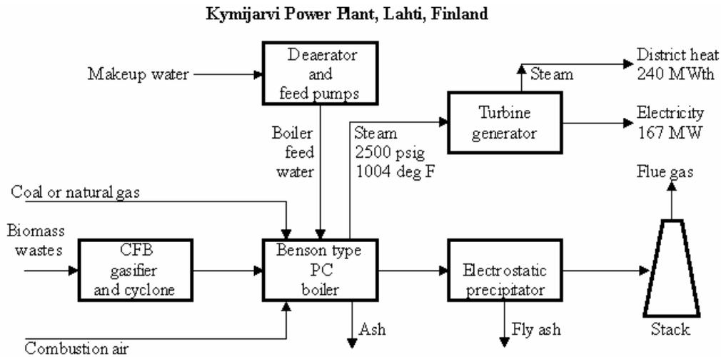
**Figure 19. Flow Diagram for the CFB gasifier at Lahti, Finland**
