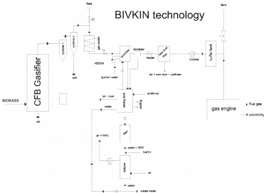
**Figure 1. Process Diagram of the BIVKIN Gasification Technology (Van der Drift et al., 2000)**
