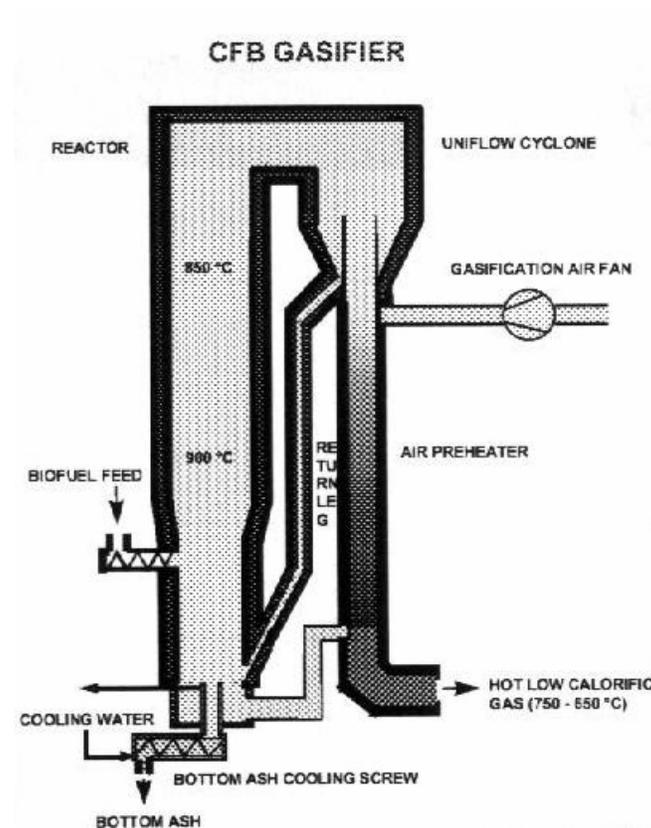
**Figure 18. Foster Wheeler's Pyroflow ACFB Gasifier**
