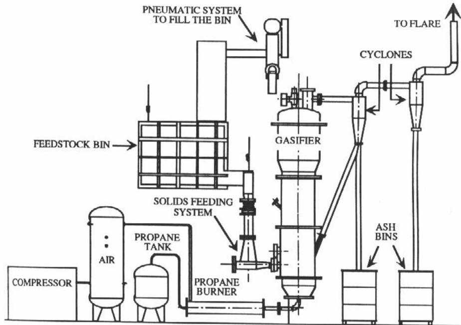
Figure 1. Process flow diagram of the gasifier installation having a nominal capacity of 500 kg/h of biomass.
