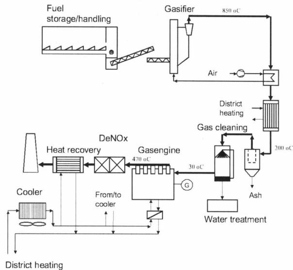
**Figure 3. Flow sheet of the 5 and 12.5 MW<sub>th</sub> BIVKIN-based power plant**
