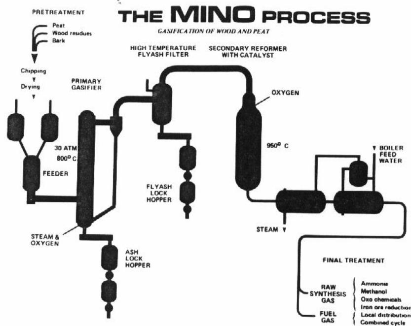
Figure 11. The MINO Gasification Process
