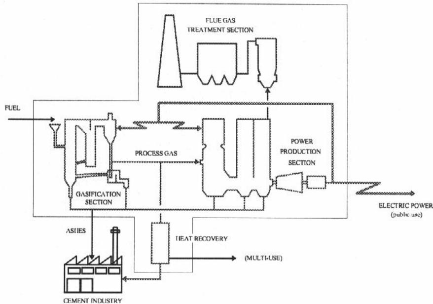
**Figure 14. Flow Diagram of the TPS Gasification System for RDF in Grève-in-Chianti, Italy**
