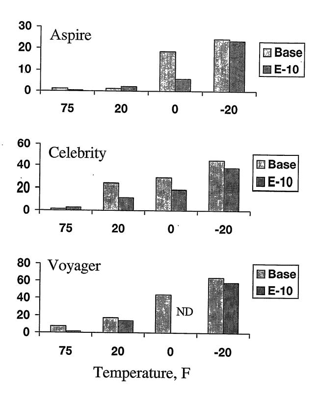
Figure 3. IM240 PM-10 Emission Rates From In-Use, High HC and/or CO Emitting Vehicles
