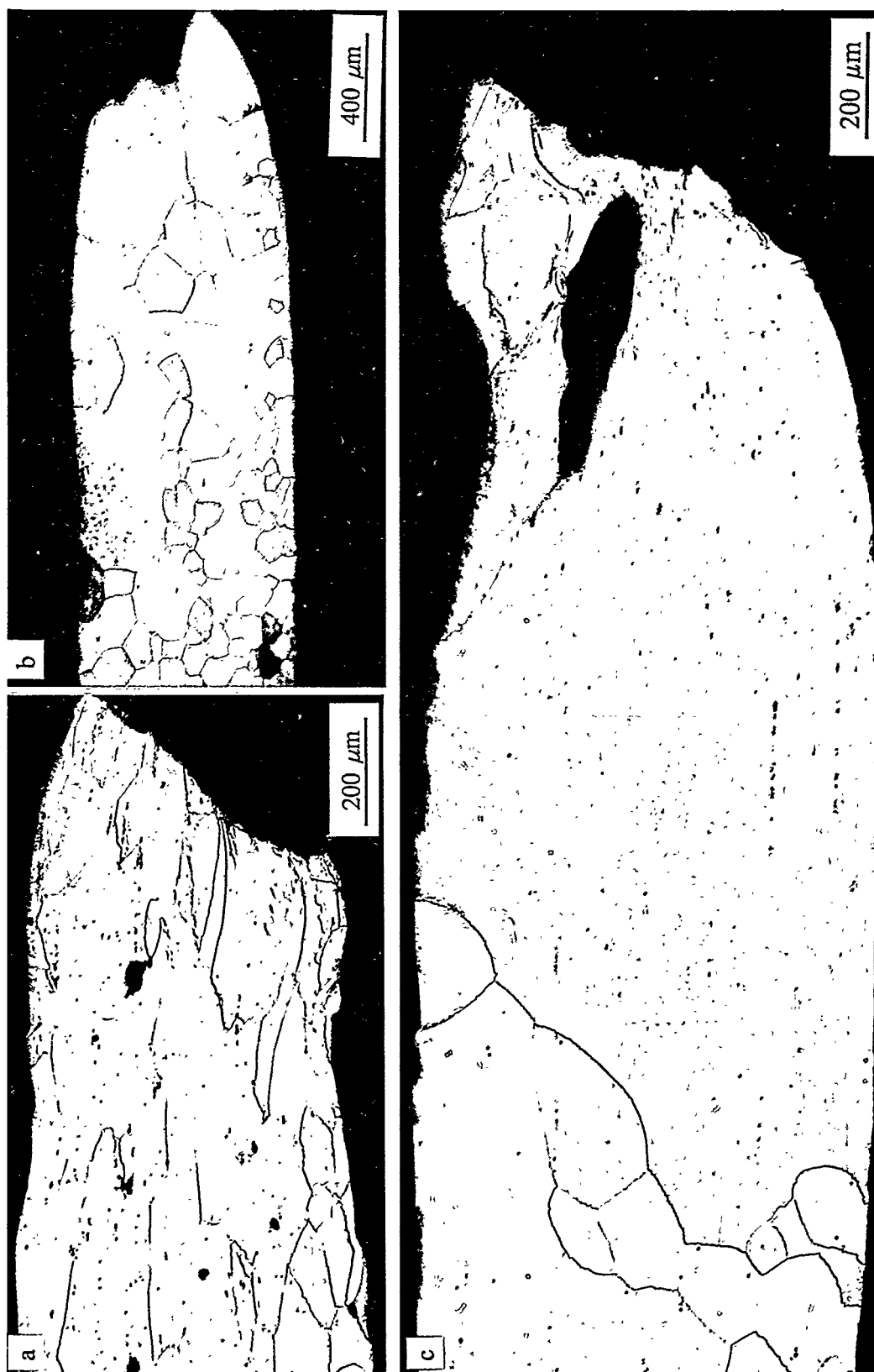
Fig. 5. Optical micrographs showing the microstructure at the fracture of specimens heat treated at (a) 1100, (b) 1175, and (c) 1225°C and tested at 593°C.
