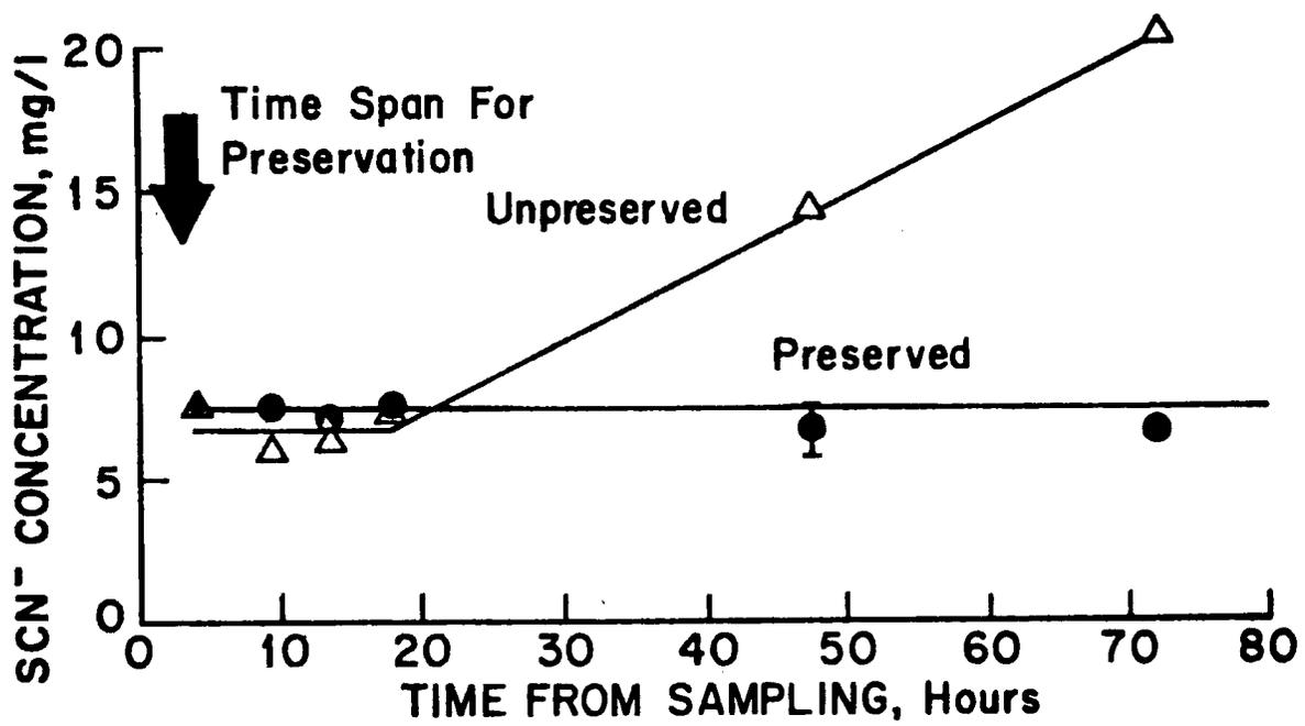
Figure 3. Time stability of cyanide and thiocyanate in preserved and unpreserved samples of gasifier quenchwater:  $\text{CO}_2$ -acceptor run 42.
