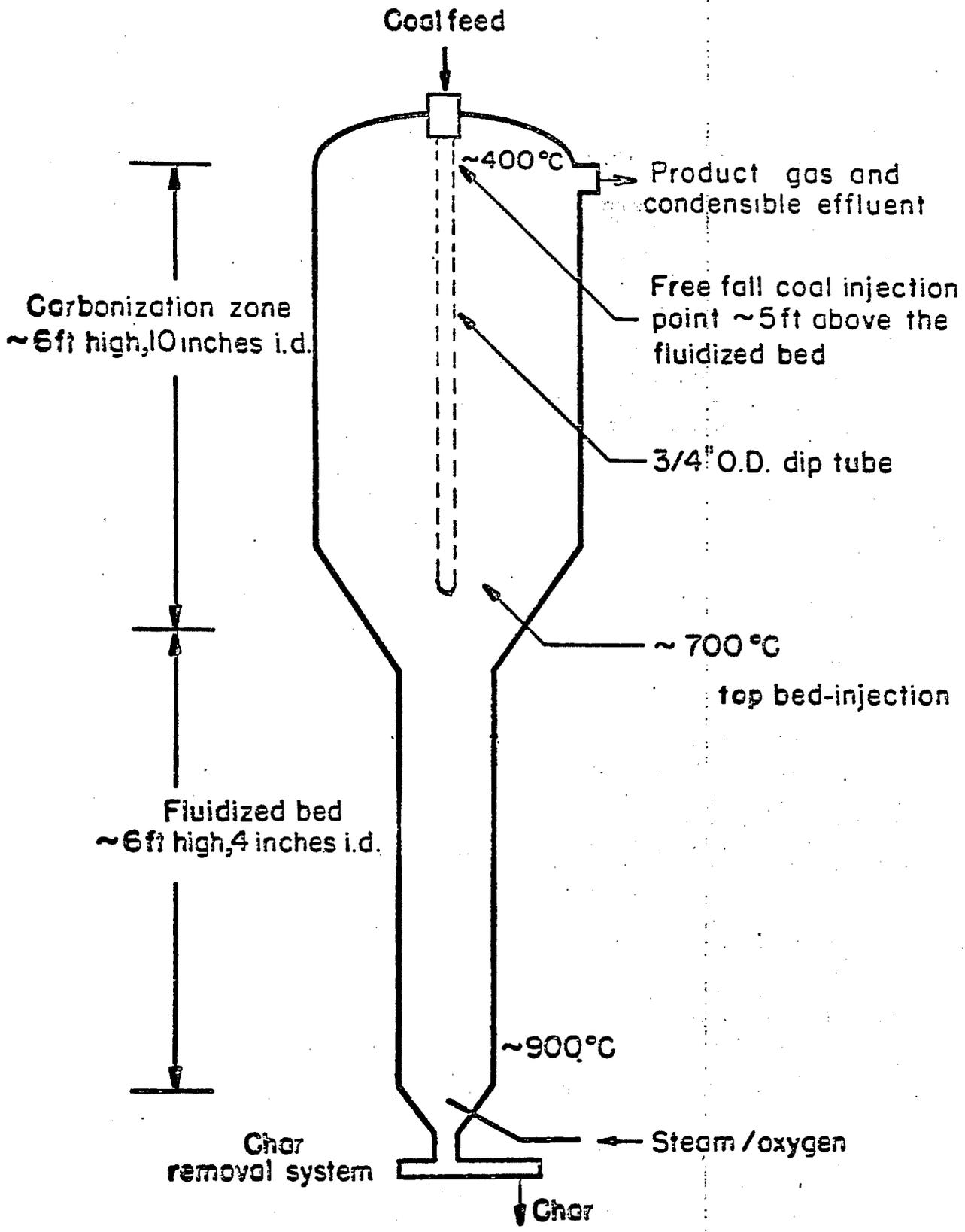
Figure 10. Synthana PDU gasifier: top bed-injection of feed coal.
