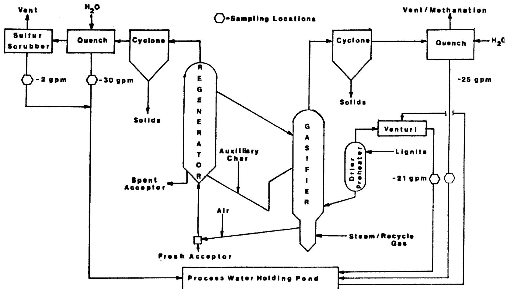
Figure 4. Liquid effluent flow patterns of the CO<sub>2</sub>-acceptor coal gasification pilot plant.
