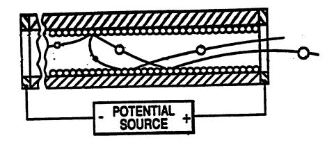
Figure 1a. Electronic conversion of methane by electron-impact reduction, electron-stimulated desorption of ions, and ion-impact-stimulated chemical combination and desorption at inside surface of a single tubular microchannel.
