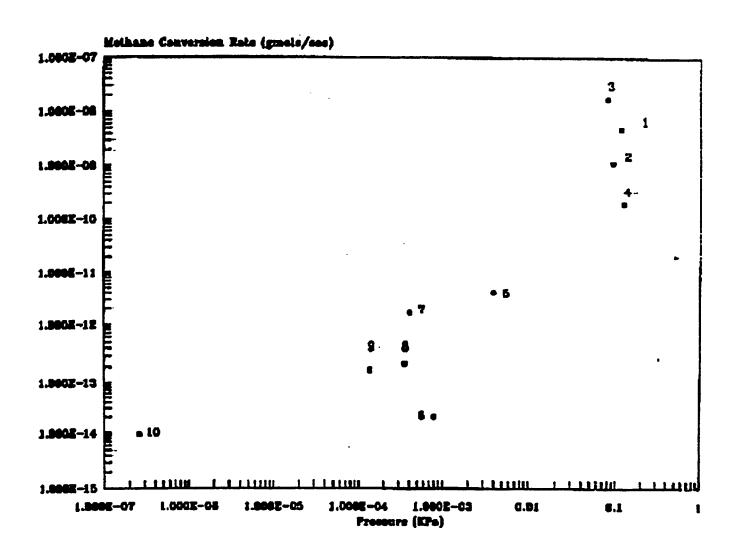
Figure 3. Log-log plot of methane conversion rate (gram-moles/second) vs. pressure, for ten experiments, showing a nonlinear increase in conversion rate as pressure increases, which is attributed to the increasing effect of ion interactions with the surface.
