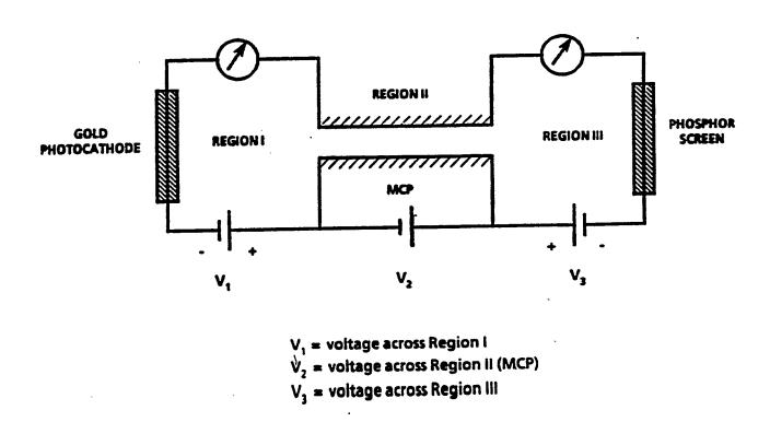
Figure 1b. Electrical circuit arrangement for methane conversion using microchannel plate (MCP) channel array.
