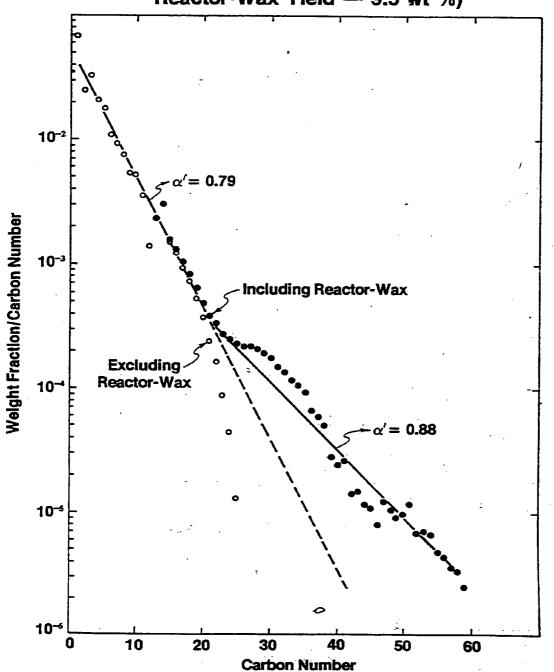
8 EFFECT OF REACTOR PRESSURE ON REACTOR-WAX CARBON-NUMBER DISTRIBL 1.48 2 DOS o **52** (Run CT-256-3) 20 SLIDE # 11 0 ဓ္ဗ Wt % of Reactor-Wax
