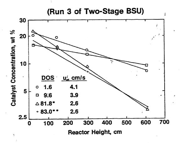
Estimated Cat. Load: 10.8-12.9 wt % Estimated Expanded Slurry Height: 610-762 cm
