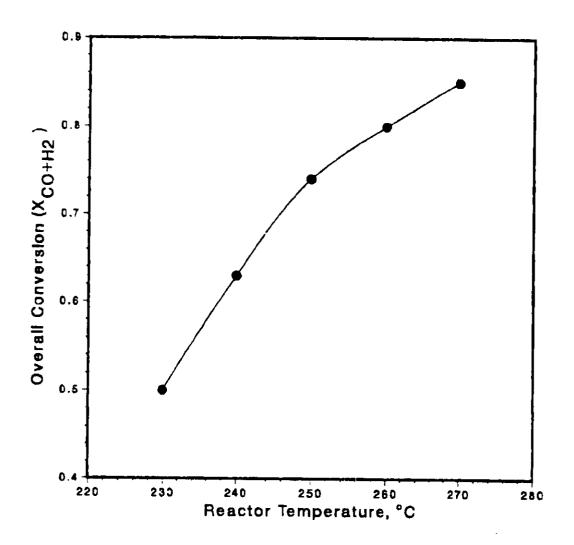
Figure 2: Effect of Reactor Temperature on Syn Gas Conversion
