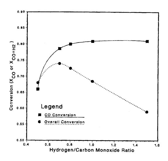
Figure 4: Effect of Hydrogen/Carbon Monoxide Ratio on Syn Gas Conversion
