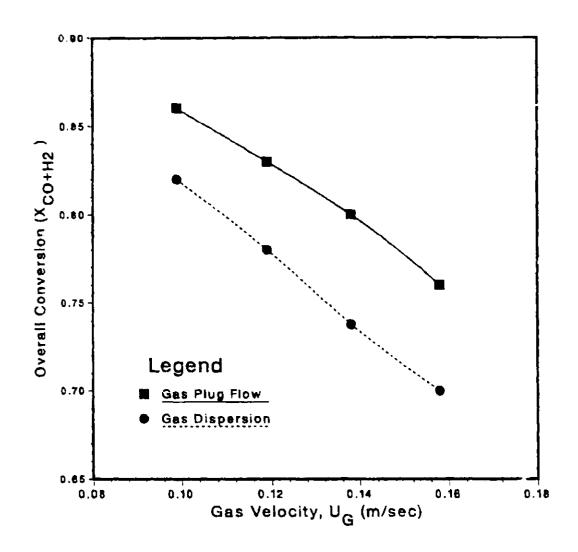
Figure 3: Effect of Gas Velocity on Syn Gas Conversion
