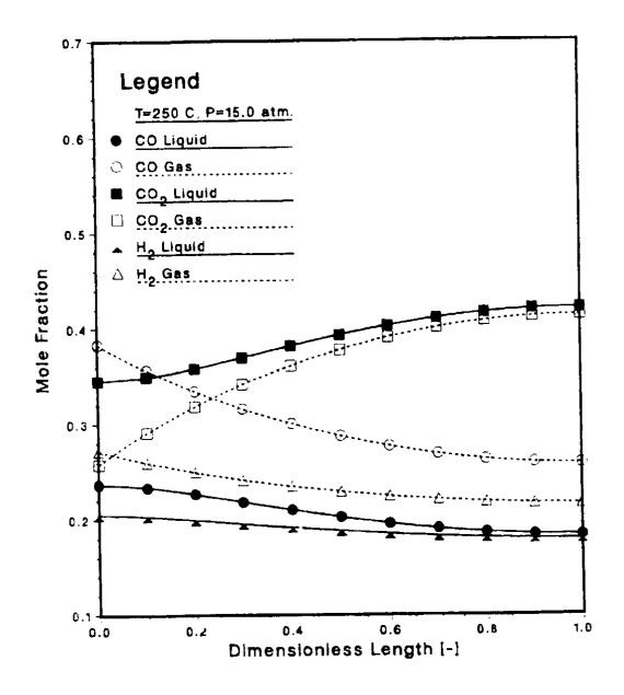
Figure 1: Concentration Profiles in Bubble Column Slurry Reactor
