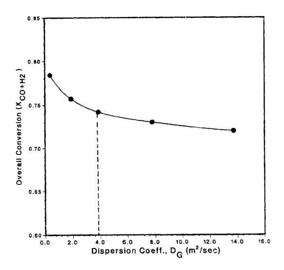
Figure 5: Effect of Gas Phase Dispersion Coefficient on Syn Gas Conversion
