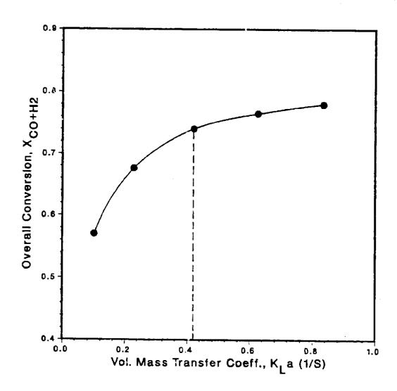
Figure 6: Effect of Volumetric Mass Transfer Coefficient on Syn Gas Conversion
