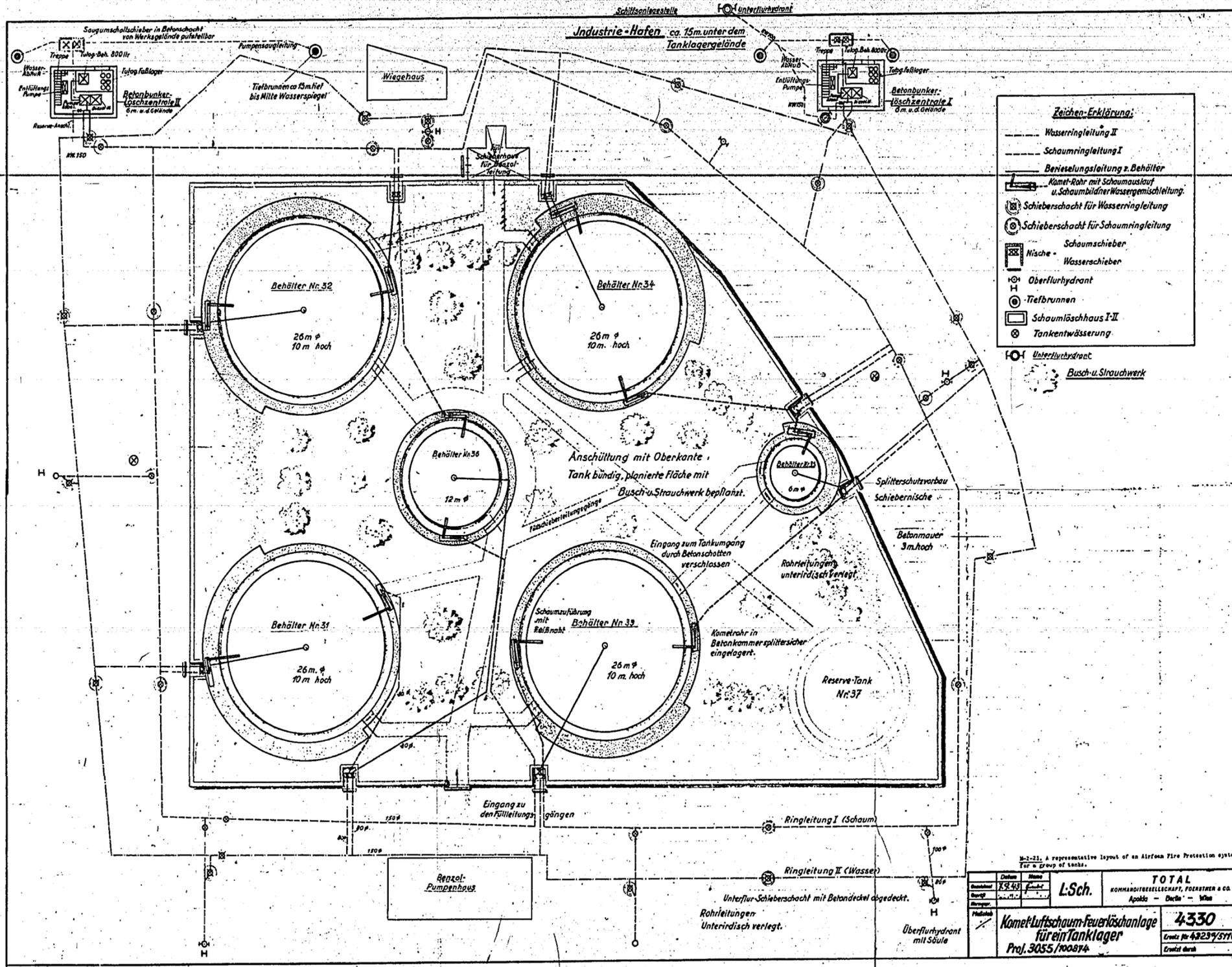
M-2-23. A representative layout of an Airfoam Fire Protection system for a group of tanks.
