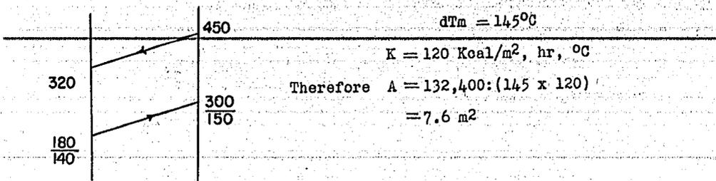
With a safety factor, the surface is  $15 \text{ m}^2$ .
