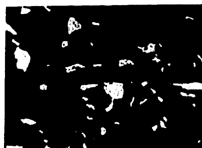
6. Al-dust with predominating leaf-like structure after 10 hours. Polished under oil.
