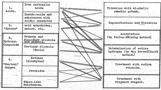
The double lines give the individual methods by which substances can actually be determined.
