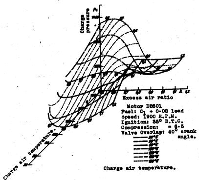
Knock limit curves of  $C_1 + 0.08$  lead with  $40^0$  valve overlap in dependence on the excess air ratio, charge pressure and charge air temperature.
