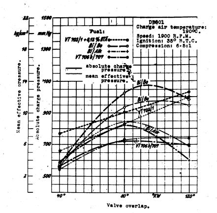
Variation of the knock resistance at the minima in the knock limit curves ( > 1.05) with change in the valve over ap at a charge air temperature of 190°C.
