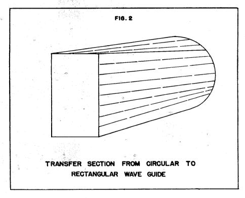
NavTechJap Document No. ND21-6232.3-1 gives dimensions of circular and rectangular wave guides and shows the construction of a transfer section.
