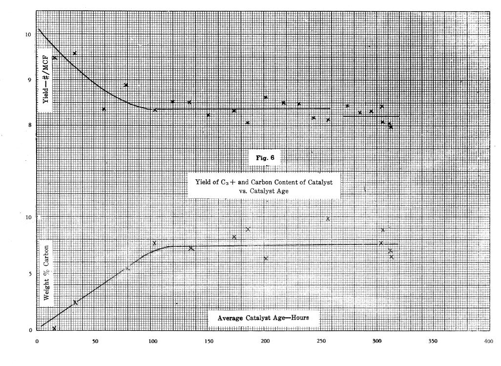
These changes are shown in the opposite Figure 6 where yield and the carbon content of the catalyst have been plotted against age. The catalyst test data are detailed in Table II, following. It should not be inferred from the plot in Figure 6 that the change in yield is necessarily a result of the change in carbon content since several other catalyst properties show similar changes during this period.
