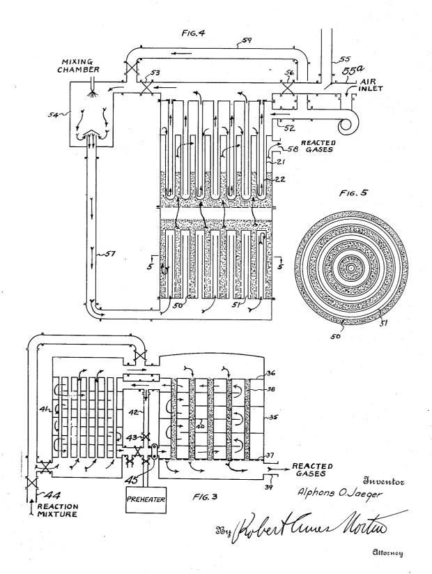
PROCESS FOR EFFECTING CATALYTIC REACTIONS
