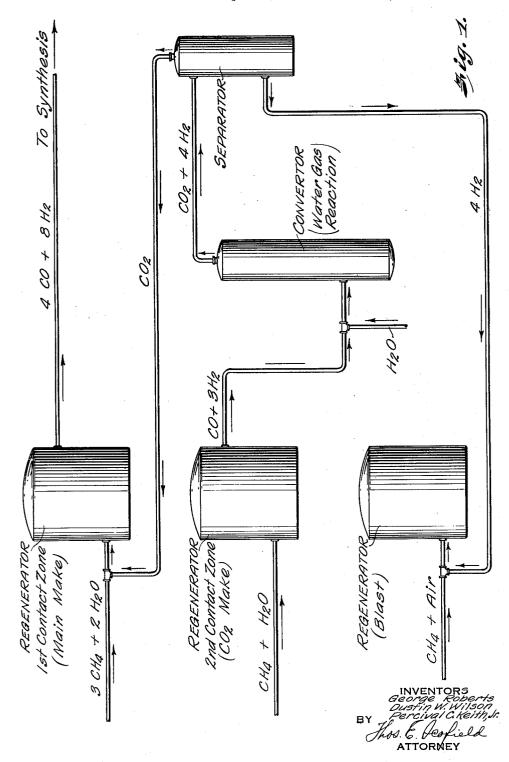
METHOD OF MAKING A SYNTHESIS GAS MIXTURE OF CARBON MONOXIDE AND HYDROGEN
