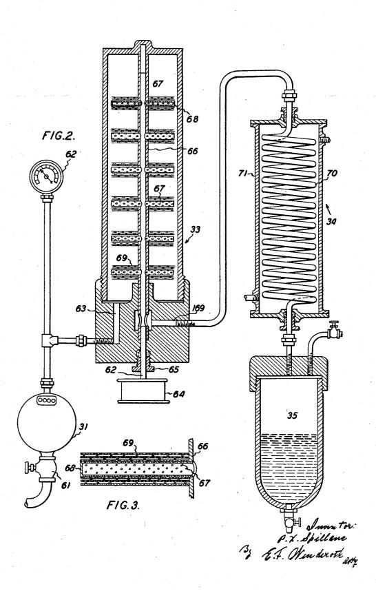
PROCESS FOR SYNTHESIS OF HYDROCARBONS ALCOHOLS AND FORMALDEHYDE
