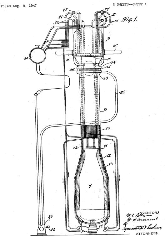
SYNTHESIS GAS GENERATOR AND WASTE HEAT BOILER
