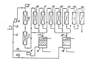
This invention relates to the production of methane containing gases and, more particularly to the production of fuel gases suitable for use as substitute natural gas (SNG) from synthesis gases obtained by the gasification of carbonaceous fuels such as oils and coal.
