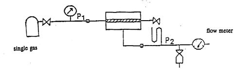
Figure 3: Reactor for gas separation of gas mixtures on microporous capillaries
