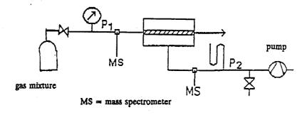
Figure 4: Reactor for gas permeation on microporous membranes
