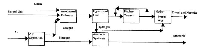
Natural gas is passed through one or more means of removing sulphur compounds from the gas so that the level of sulphur no longer poses a poisoning risk for either a Fischer-Tropsch or an ammonia synthesis catalyst. The desulfurized natural gas is then combined with oxygen and steam and reacted in an autothermal reformer. The oxygen is
