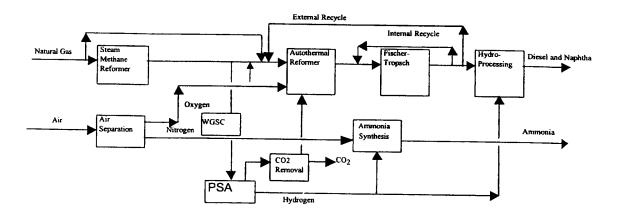
A plant of this type is used to produce 30 000 barrels per day (bpd) of liquid hydrocarbons and a further 1 000 tons per day of ammonia. Natural gas with the composition given in Table 1 of example 1 is again utilised for the purposes of this illustration. Process conditions may alter depending on the composition of natural gas in different situations. Process conditions will also alter depending on the relative quantities of ammonia and hydrocarbon products desired.
