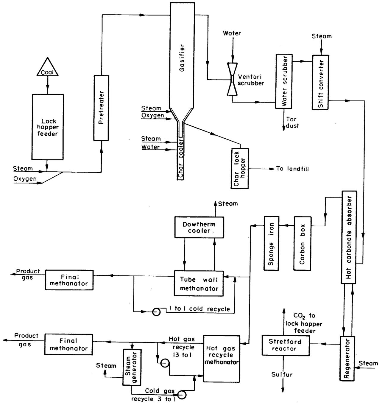
FIGURE 5. - Flowsheet of Prototype Synthane Process.
